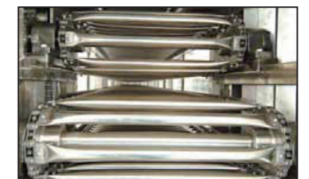
連續式熟成室內部 Continuous Noodle Dough Sheet Aging Machine-Inside Section
