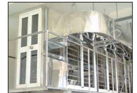
連續式熟成室後段 Continuous Noodle Dough Sheet Aging Machine-Back Section
