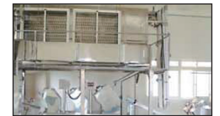
連續式熟成室前段 Continuous Noodle Dough Sheet Aging Machine-Front Section
