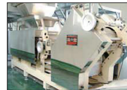
複合機 Compound Pressing Machine
