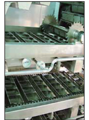
三層冷卻槽 Three-Level Cooling Tank
